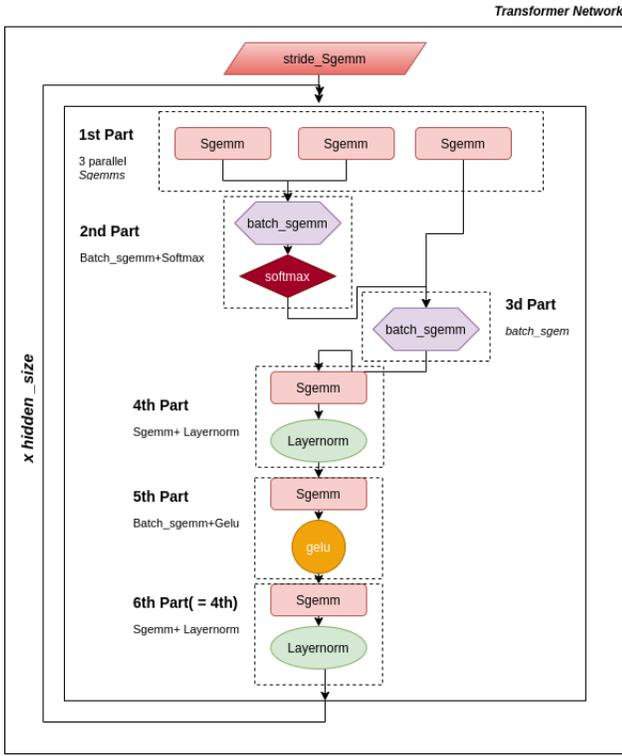
Fig. 1. FPGA Transformer Network Architecture
