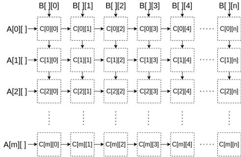
Fig. 2. Systolic array for Batch\_sgemm
