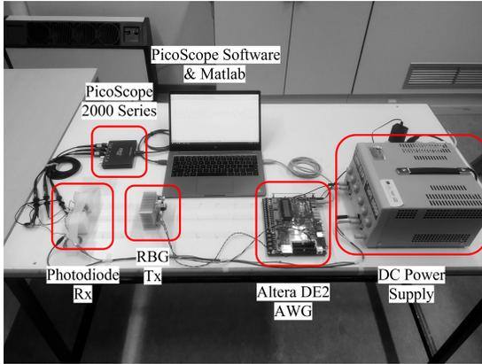
Fig. 4: The experimental setup used in the measurements.
