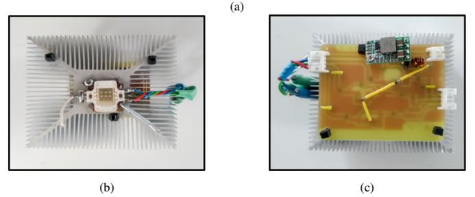
Fig. 5: (a) The LED driver for each color channel, (b) frontside and (c) backside of the implemented RGB LED transmitter.
